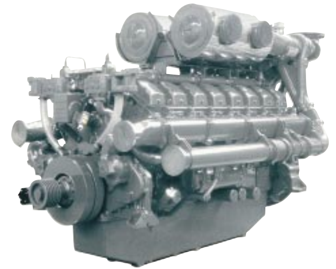
4016 16 cylinder 60° Vee form water cooled diesel engine developing 824-1886 kWm net
